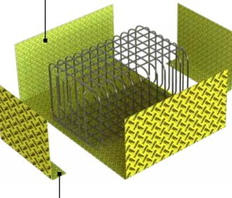
EcoBase panels are intentionally bent to prevent floating issues that may occur during foundation pouring.
